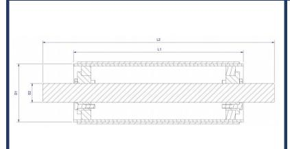
As a standard, the return drum is made of a pipe and an axle blocked with clamping sleeves that enable the adjustment of the position of the axle in relation to the drum or its replacement. Drums are painted in RAL color, optionally they can be galvanized. As standard, the drums are permanently covered with rubber, increasing their friction against the belt.
