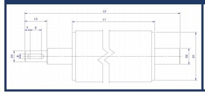
The standard equipment corresponds to the return drums and is extended by a profiled end of the axle enabling its integration with the drive unit.
