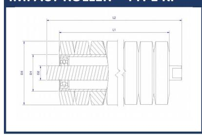
The standard equipment corresponds to a smooth roller and is extended by rubber rings made of rubber with a hardness selected by the customer, permanently glued to the roller covering its entire surface.
