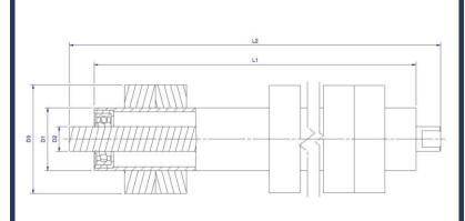
The standard of equipment corresponds to a smooth roller and is extended by rubber discs made of rubber with a hardness selected by the customer, permanently glued to the roller according to the indicated spacing
