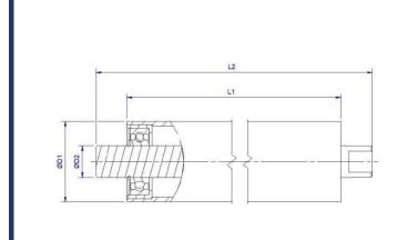
The smooth roller is equipped as standard with high-quality double-sided covered bearings mounted in turned housings welded into both ends of the pulley. Standard anti-corrosion protection is hot-dip galvanizing. optionally it is possible to equipt the roller with an additional labyrinth seal and paint it on a color of your choice.
