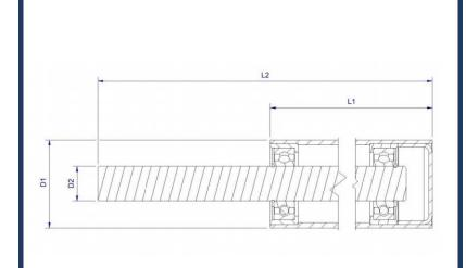
The standard directional roller is equipped with high-quality bearings covered on both sides, mounted in turned housings welded at both ends. The standard anti-corrosion protection is hot-dip galvanizing. It is possible to equip the roller with an additional labyrinth seal and paint it with a selected color. As a standard, the directional roller has one of the ends plugged in a way that allows its disassembly
